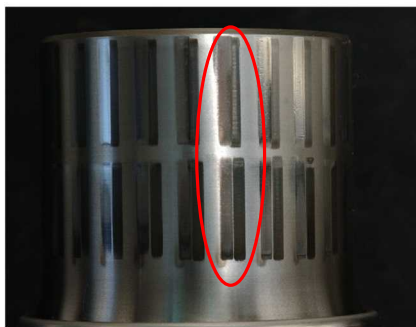
Figure 14 Examples of damage to rolling surface of cross pin
