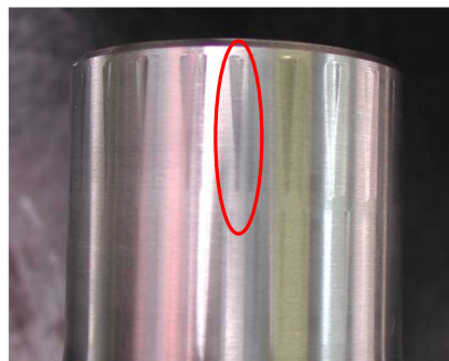
Figure 14 Examples of damage to rolling surface of cross pin
